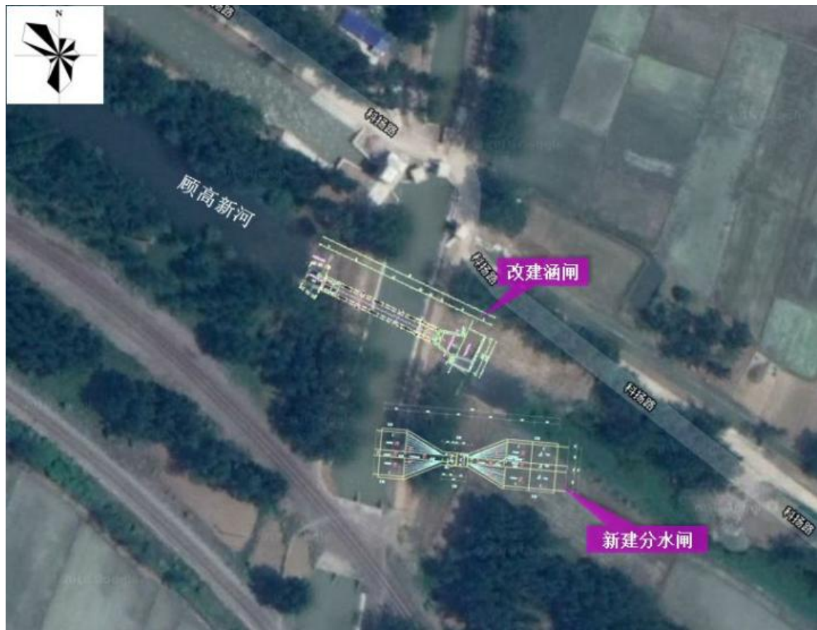
图 3.3.3-3 架河灌区总干渠新建分水闸与顾高新河改建涵闸
